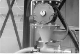
From the point of view of the operational flow, the injection system had to be connected to a pneumatic system installed in the area ATEX 22, therefore had to be designed and constructed with suitable characteristics. The most immediate solution would be to provide for all ATEX certified machines, then certify entire system. In this occasion our design activity has set the goal of containing the of while costs supply, maintaining compatibility with the system requirements.
